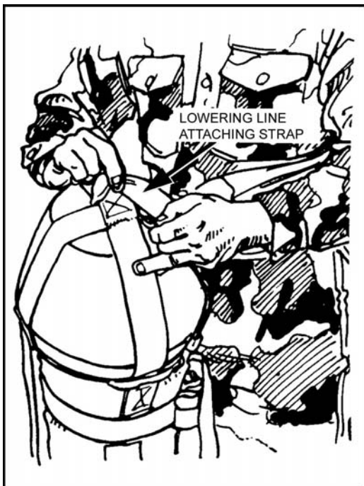
Figure 12-35. Lowering line attaching strap installed.
